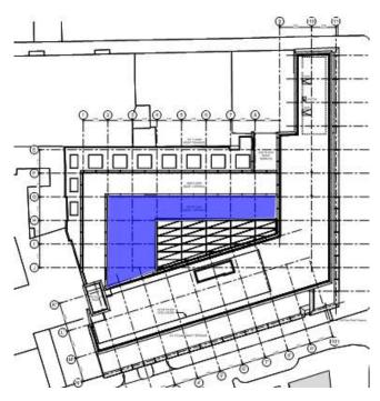
Although almost 100m2 of green roof, at variable depths, has been retained in the design this is insufficient to provide the level of attenuation required to achieve the 50% reduction in flows required for the building.
