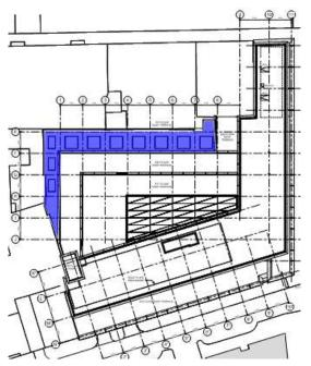
This roof has been detailed by the Architect / Landscape architect to be able to be the primary area for rooftop attenuation along with the Level 8 roof.
