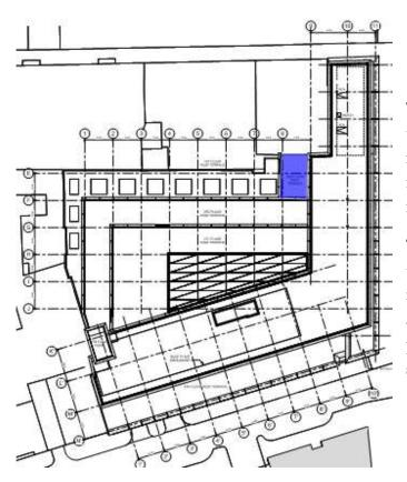
There is approximately 26m2 of green roof at this level, at variable depths, This is considered insufficient to provide the level of attenuation required to achieve the 50% reduction in flows required for the building.
