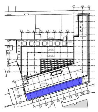
This roof area has two distinct zones. The planted zone has the ability to hold water for attenuation, whilst the zone closest to the level threshold into the building is of insufficient depth to facilitate this.
