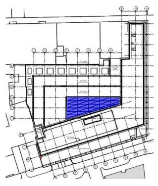
This glazed roof has no potential for attenuation. The roof will be provided with a continuous perimeter gutter. External rainwater pipes will collect the water and route it to the Level 4 roof from where it will cascade and become part of the attenuated flow at Level 1.
