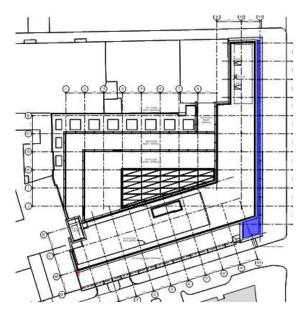
The green rood portion of this roof has been removed and therefore the rainwater discharges traditionally to the gravity system.
