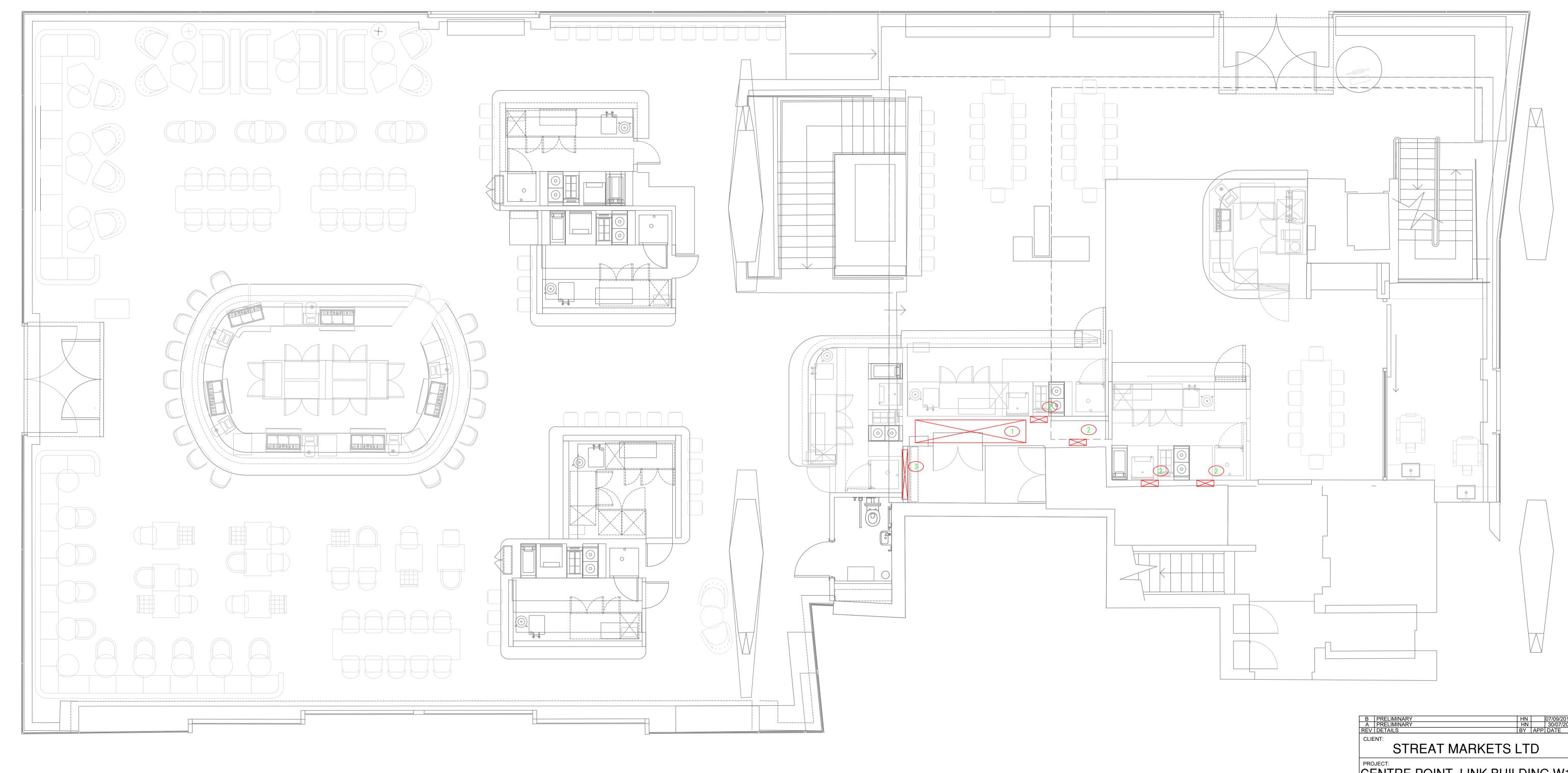
3000x600 OPENING IN FLOOR, FOR SUPPLY AIR DUCT AND KITCHEN EXTRACT DUCT
