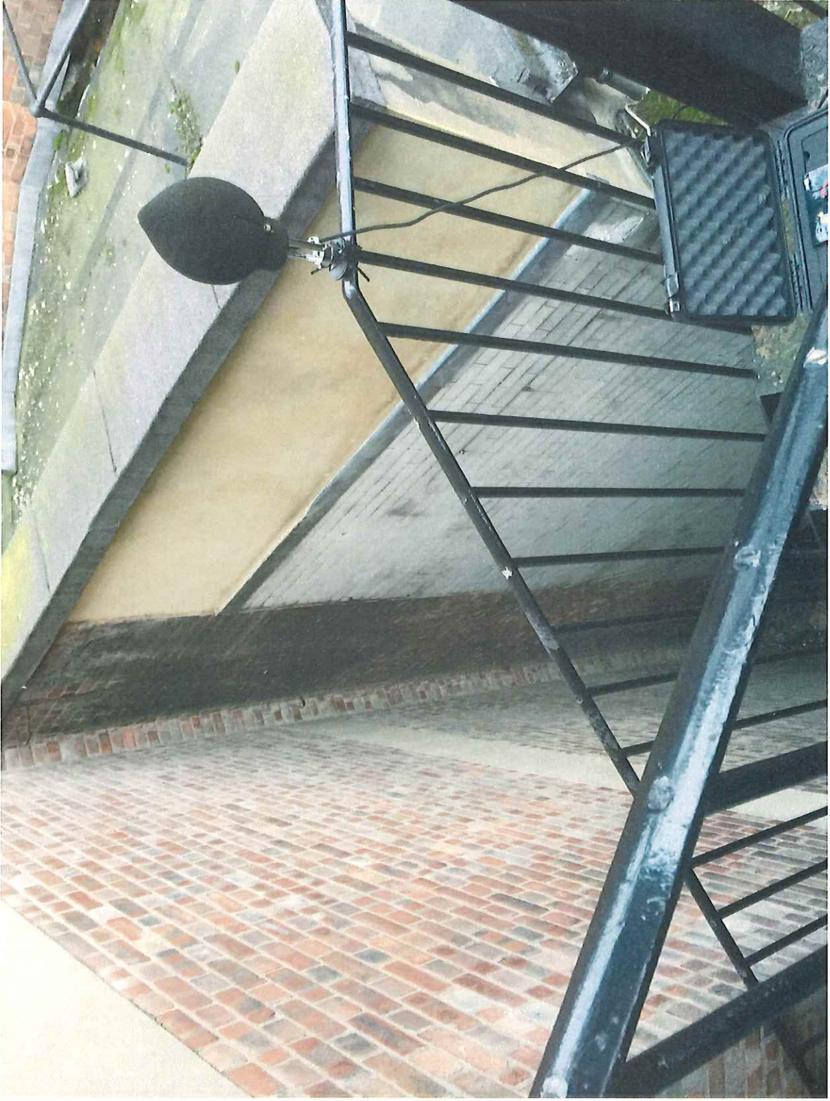
Photo E – Location of Microphone Strapped to staircase railings at 4 th Floor Level
