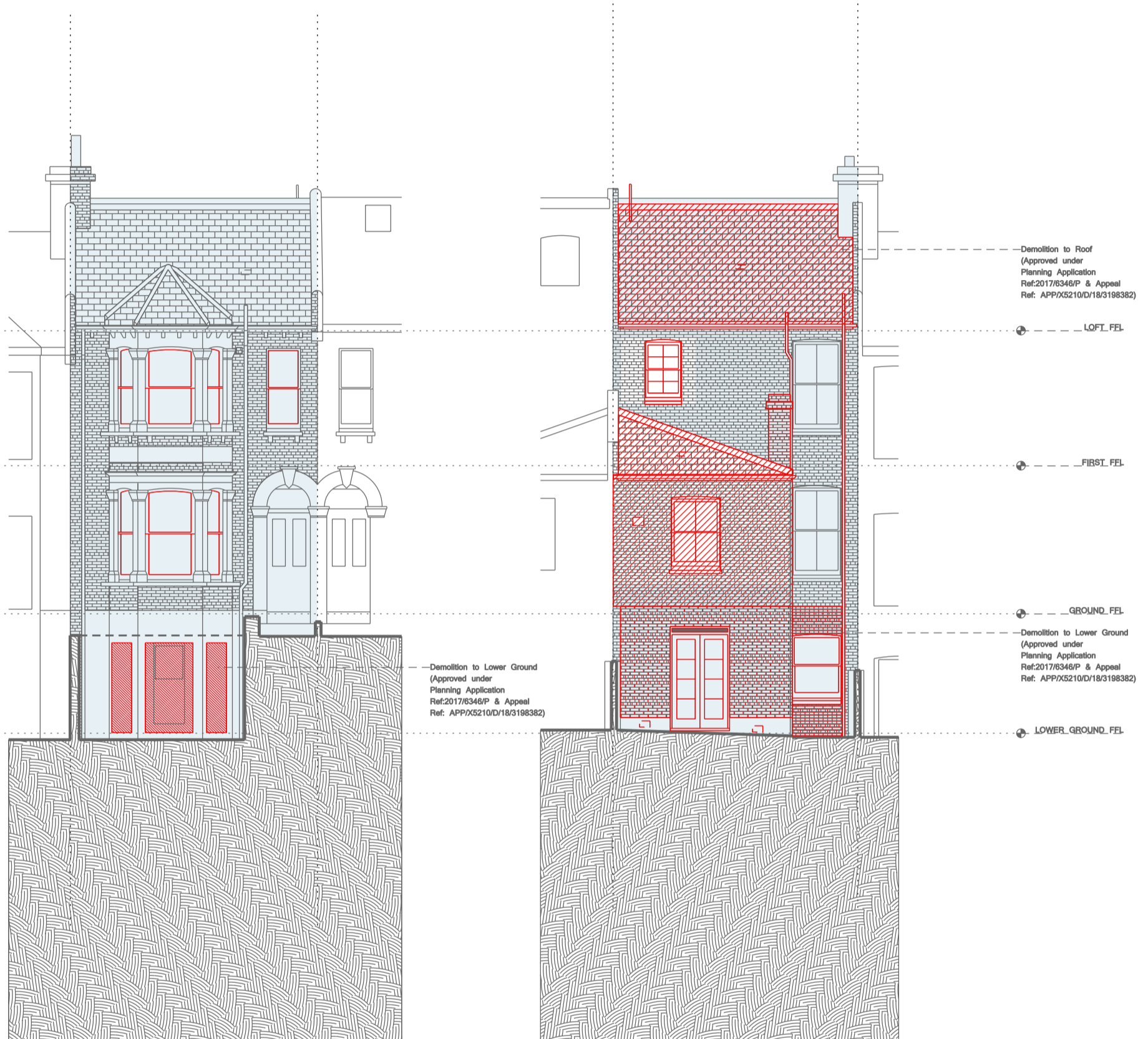
DEMOLITION ELEVATION Y1
