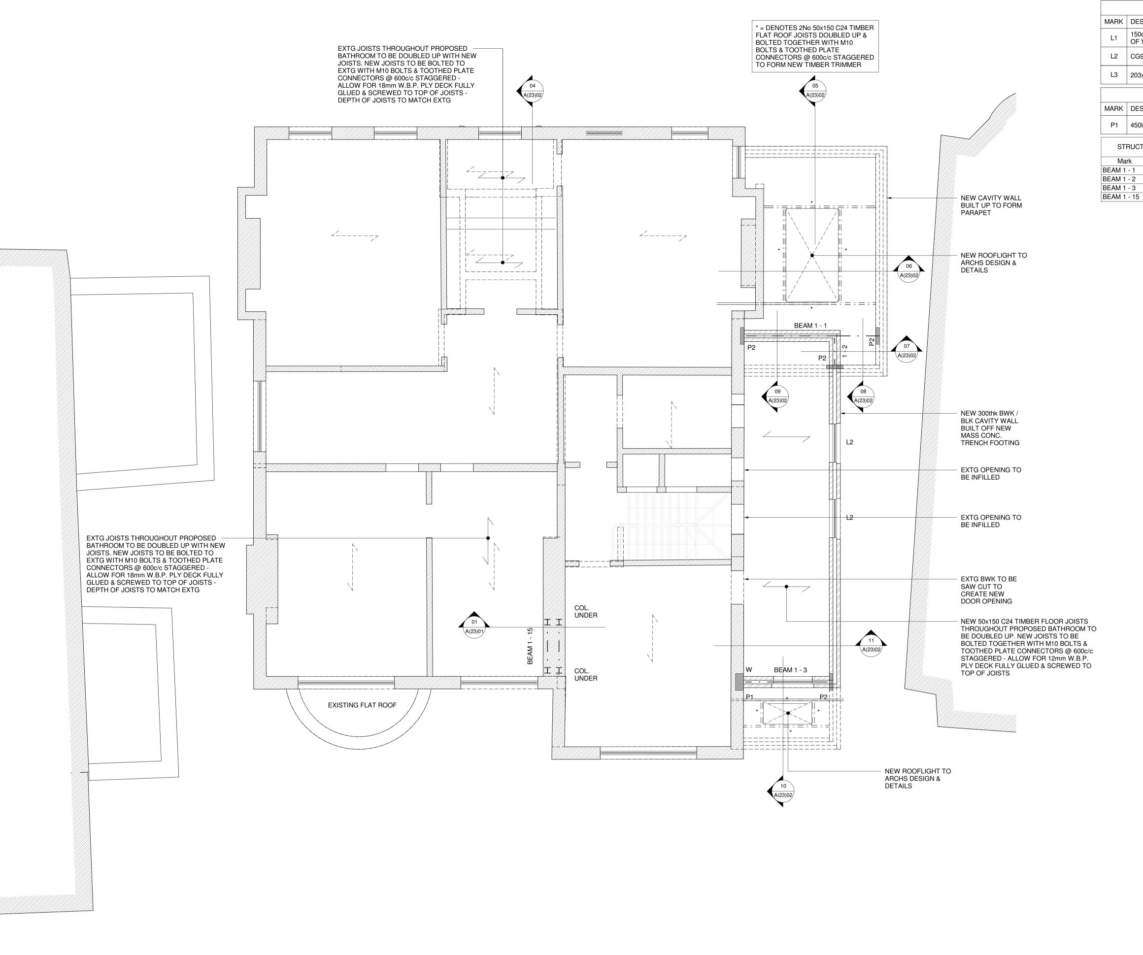
LINTEL SCHEDULE MARK DESCRIPTION 150dp PRE-STRESSED P.C LINTEL/S TO SUIT WIDTH OF WALL CG90/100 CATNIC CAVITY WALL LINTEL L3 203x203 UC60 PADSTONE SCHEDULE MARK DESCRIPTION P1 450lgx225dpxWIDTH OF WALL MASS CONCRETE STRUCTURAL FIRST FLOOR STEEL BEAM SCHEDULE Mark BEAM 1 - 1 UC152x152x37 + 15mm WELDED TOP PLATE BEAM 1 - 2 UC152x152x37 + 15mm WELDED TOP PLATE BEAM 1 - 3 UC152x152x37 + 15mm WELDED TOP PLATE
