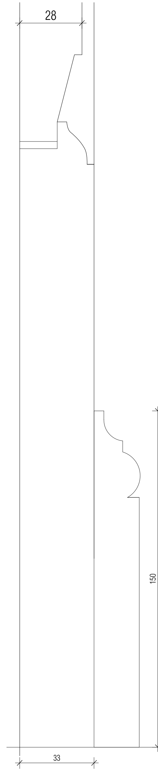
SP04 Skirting Profile 4 (the same profile as per SP07, but to be pine) (pg.170; item 1; No.15 Elder Street; 1727)
