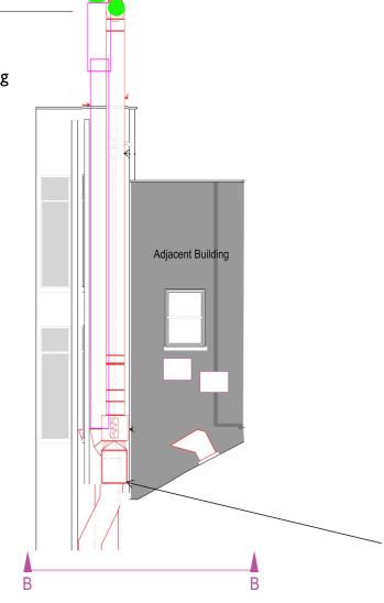
existing seperate kitchen fans with new attenuators added
