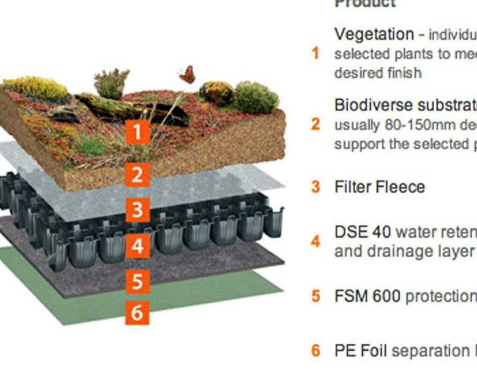
3D Sectional Diagram of Roof Build Up of Flora 3/UK Native British Provenance Seed Mix
