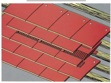
Generous 7500mm<sup>2</sup> airflow enables them to be widely spaced. Simple to fit without the necessity for cut battens or tiles.
