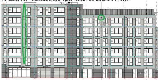
Any intakes on the railway side should be relocated to the least polluted available points. The chosen locations should take account of the predominant wind direction and dispersion patterns, and this should be demonstrated.
