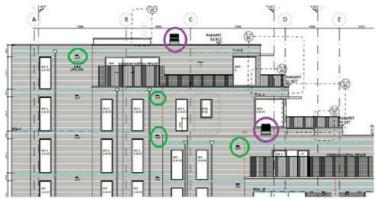
Any and all intakes which may be affected by downward or upward plumes from boiler stacks should be relocated to the least polluted available position.
