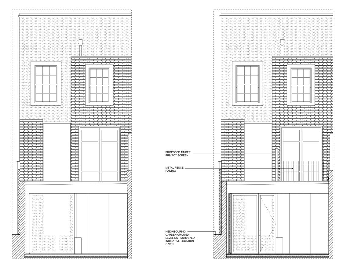
01 EXISTING REAR ELEVATION 08-802 1:50 @ A3 02 PROPOSED REAR ELEVATION 08-802 1:50 @ A3
