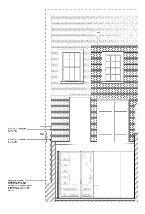
01 EXISTING COURTYARD SECTION AND REAR ELEVATION 02-100 1:50 @ A3
