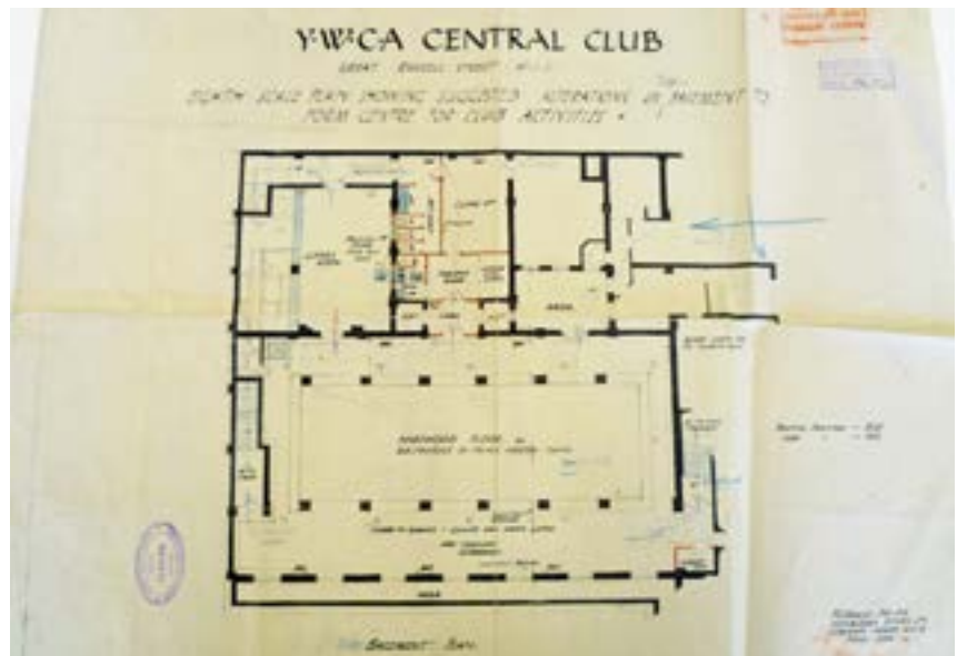
Plate 9 Basement Alterations, includes flooring over swimming pool, 1936 (LMA)
