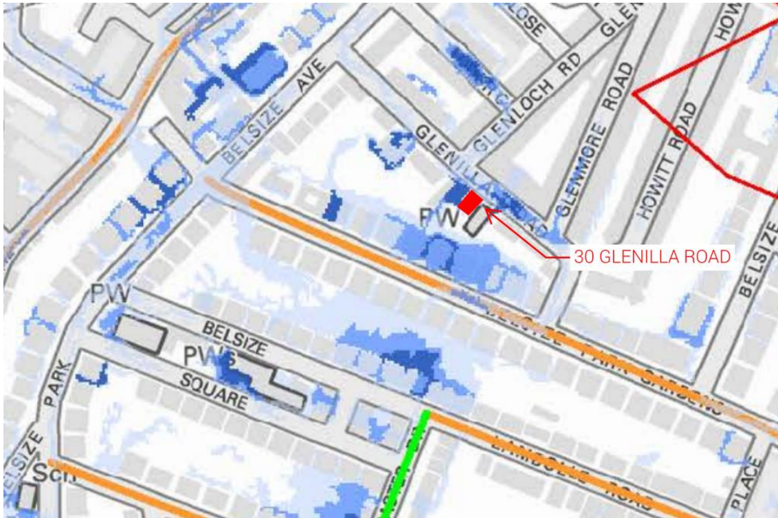
Figure 14 – Extract from Updated Flood Risk for Surface Water Flooding in the Camden SFRA
