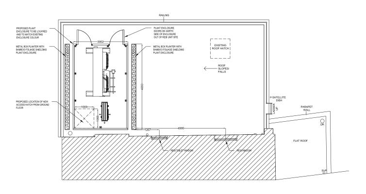
PROPOSED ROOF PLAN (Scale 1:50@ A1)
