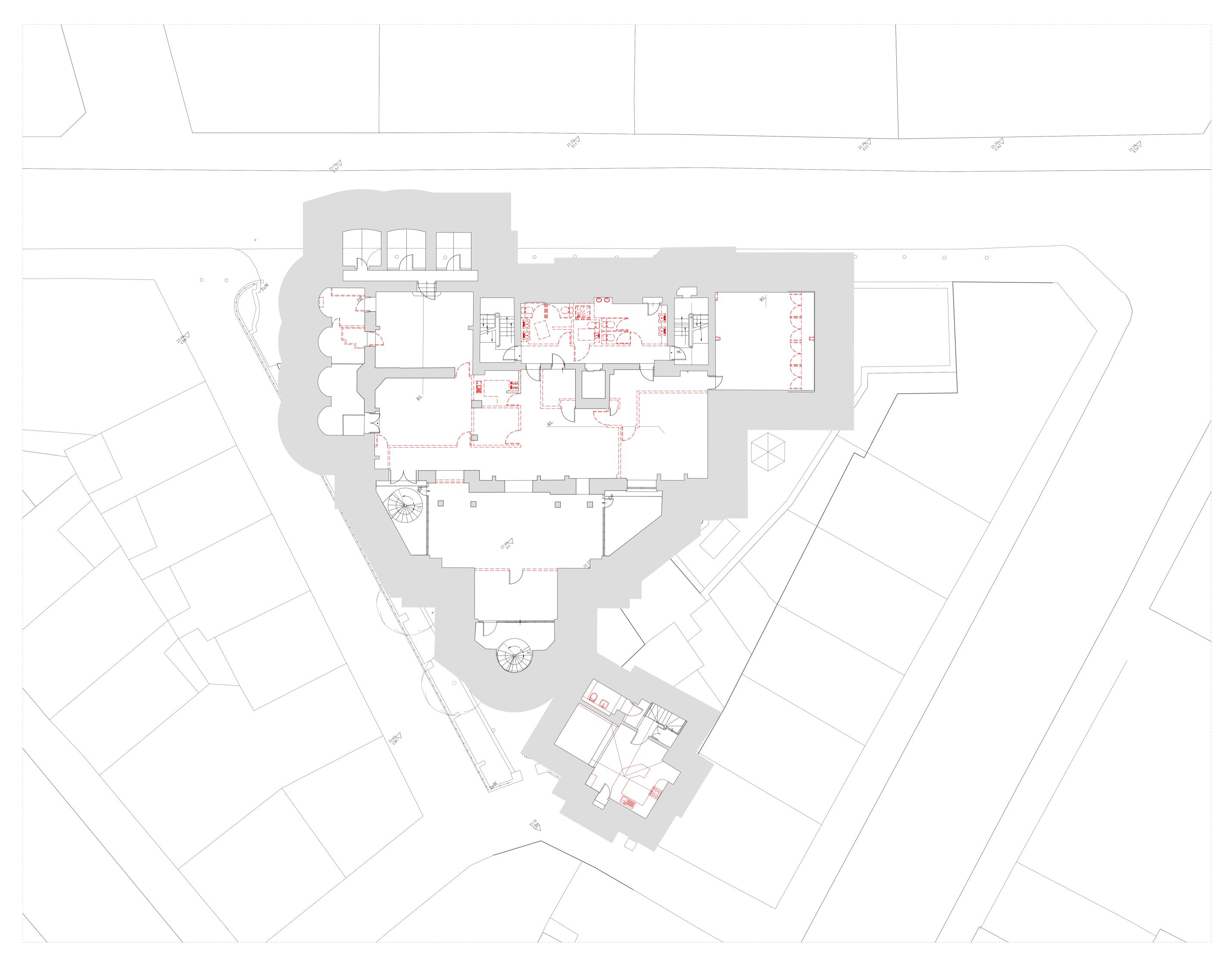
ALL NON-ORIGINAL NON-LOADBEARING PARTITIONS TO BE REMOVED ALL NON-ORIGINAL DOORSETS TO BE REMOVED ALL NON-ORIGINAL FLOOR AND CEILING FINISHES TO BE REMOVED
