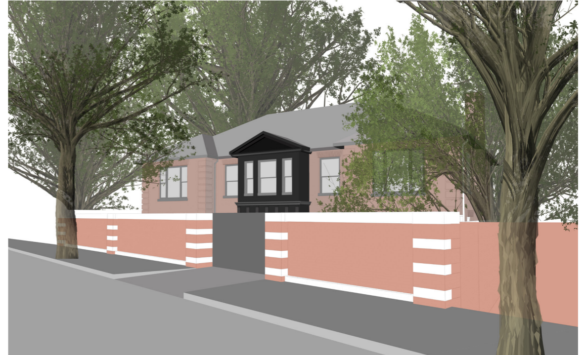
Front elevation as it would look (2017/5946/P) - hipped roof additions and natural stonework to central bay (black granite) - 3D sketch render - Above.
