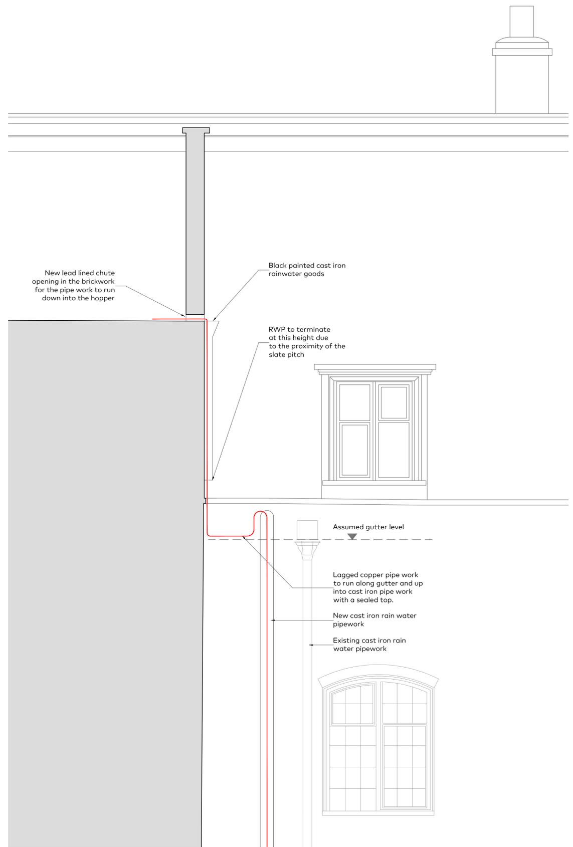
01 - Pipe drop from Plant Area No.2 to serve basement and ground floor unit
