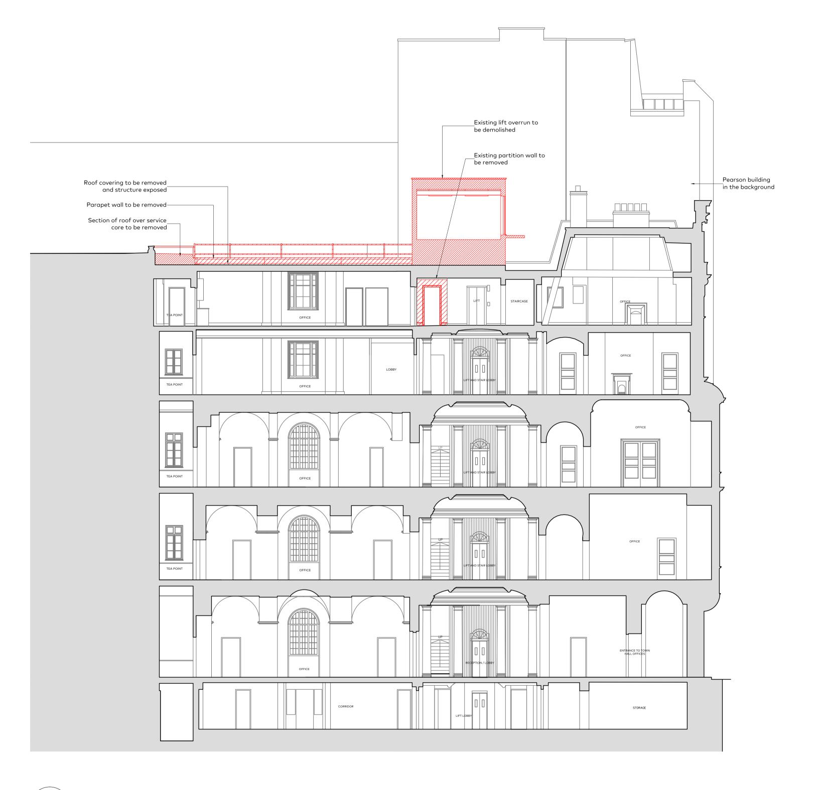
SECTION A-A As Existing with Demolitions
