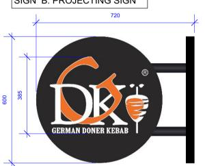
INTERNAL ALUMINIUM FRAME-LIGHT SHEET. TRANSLUCENT ORANGE VINYL TO FACE FRET CUT BACK TO BACK TRAYS 5mm THICK 050 ACRYLIC CARRIER PANEL
