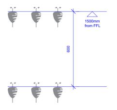
SIGN C - SIGNAGE CONTRACTOR TO SUPPLY & INSTALL NEW INTERNALLY APPLIED VINYL MANIFESTATIONS TO REFER TO DWG No 391-E:02 FOR EXTENT OF APPLICATION
