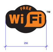
SIGN F- SIGNAGE CONTRACTOR TO SUPPLY & INSTALL NEW INTERNALLY APPLIED WINDOW VINYLS AS DWG 391-E:02
