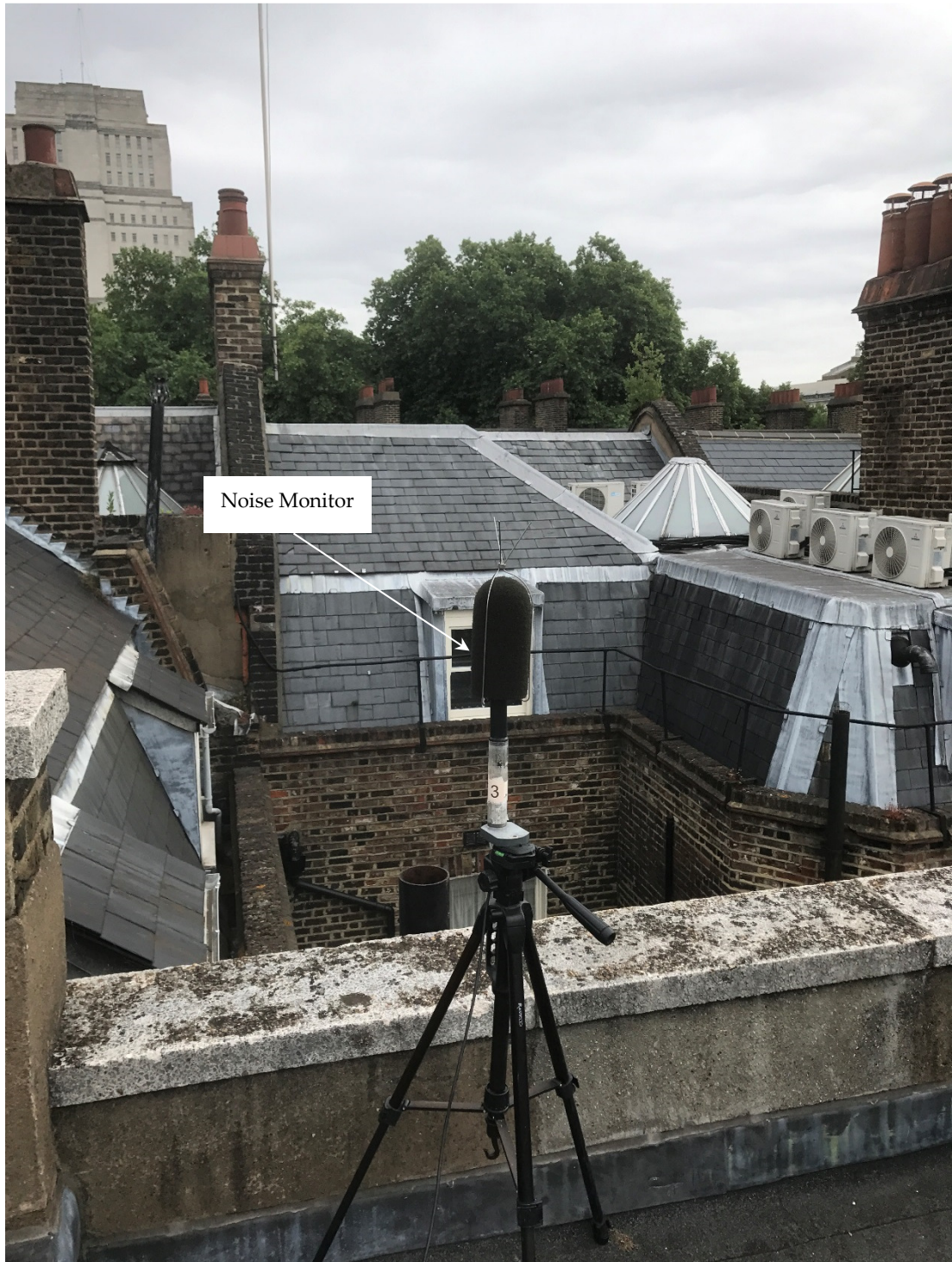
Figure A2: Noise Monitoring Equipment on the roof at 41 Store Street
