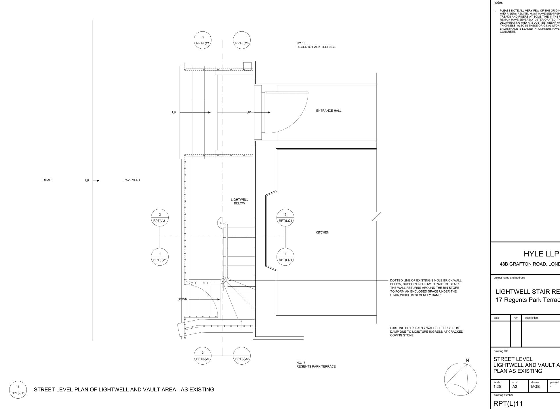
PLEASE NOTE ALL VERY FEW OF THE ORIGINAL YORK STONE TREADS AND RISERS REMAIN. MOST HAVE BEEN REPLACED BY CONCRETE TREADS AND RISERS AT SOME TIME IN THE PAST. THOSE THAT DO REMAIN HAVE SEVERELY DETERIORATED. THE STONE IS
