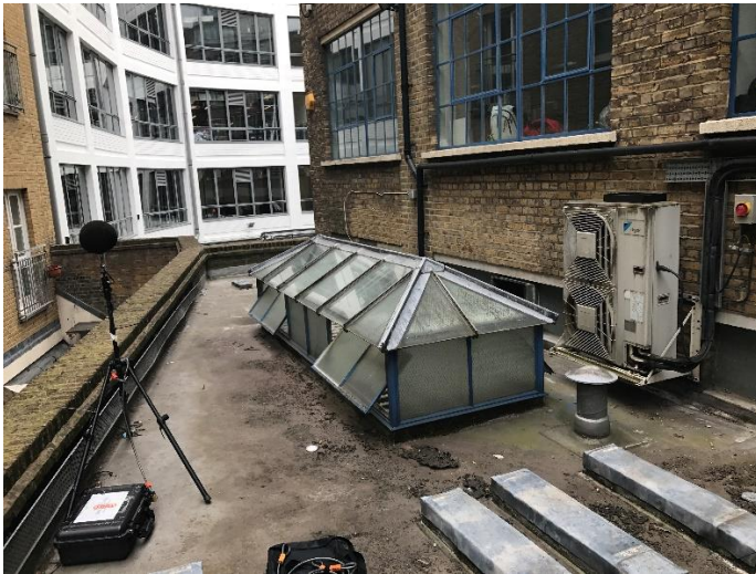
Figure 3 Photograph showing unattended noise logger position
