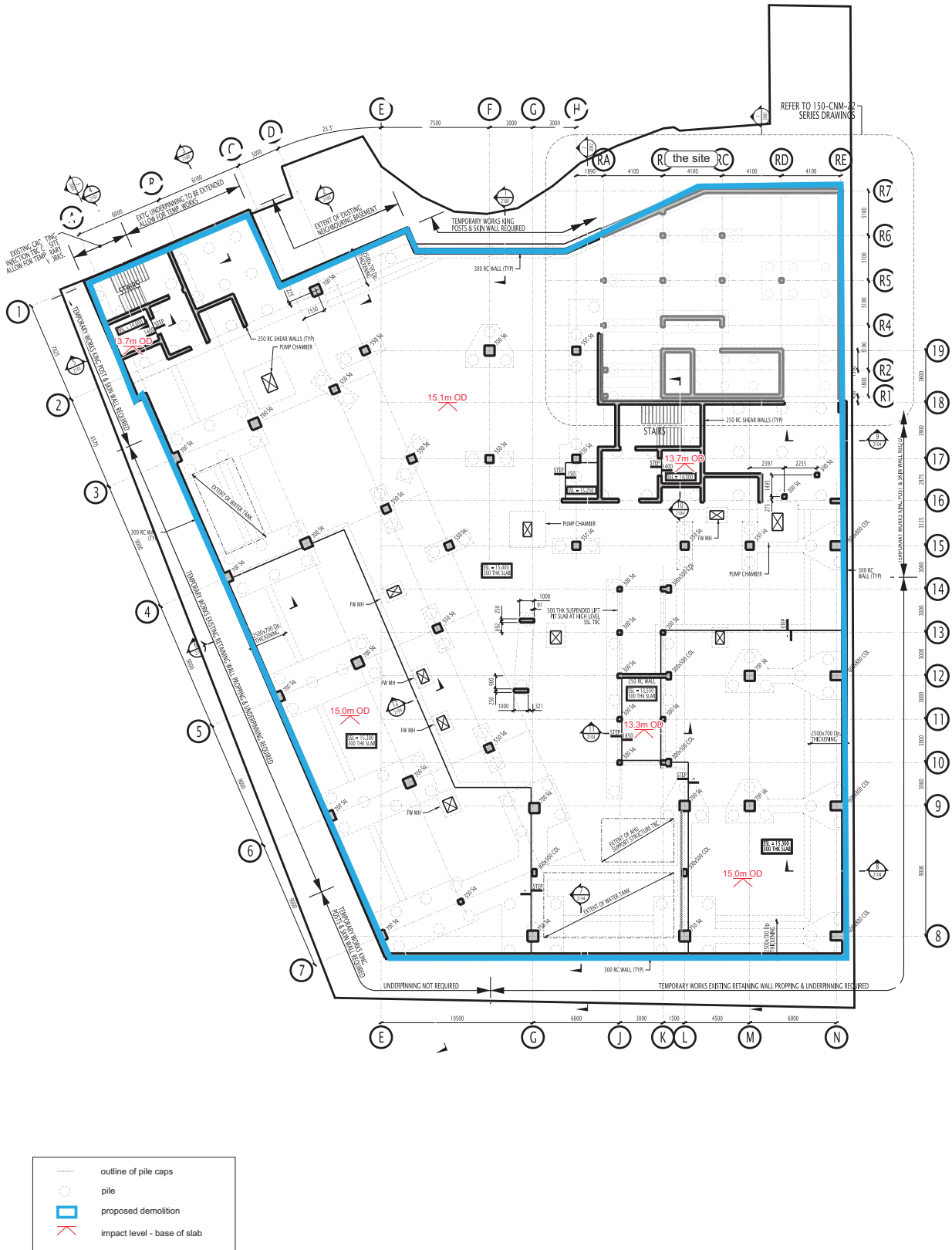
Fig 2 Existing Basement plan showing pile caps and piles below (Perkins + Will, 150-CNM-Z1-B1-DR-S-1012, Rev P1.04, 07.09.2017)
