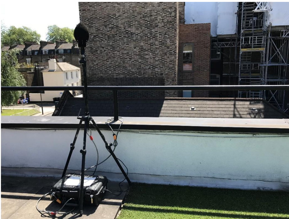
Figure 2 Noise monitor on site
