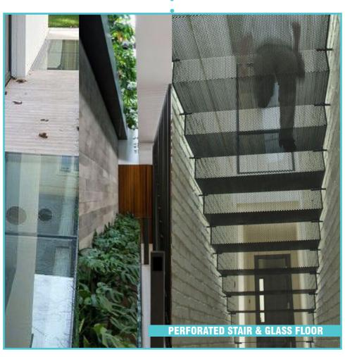
The front light well provides access as well as light and ventilation to the lower ground floor. A structural perforated metal stair will allow light penetration whilst planted interior walls will create visual interest. A glass block floor will allow diffused light into the conference spaces at basement level.
