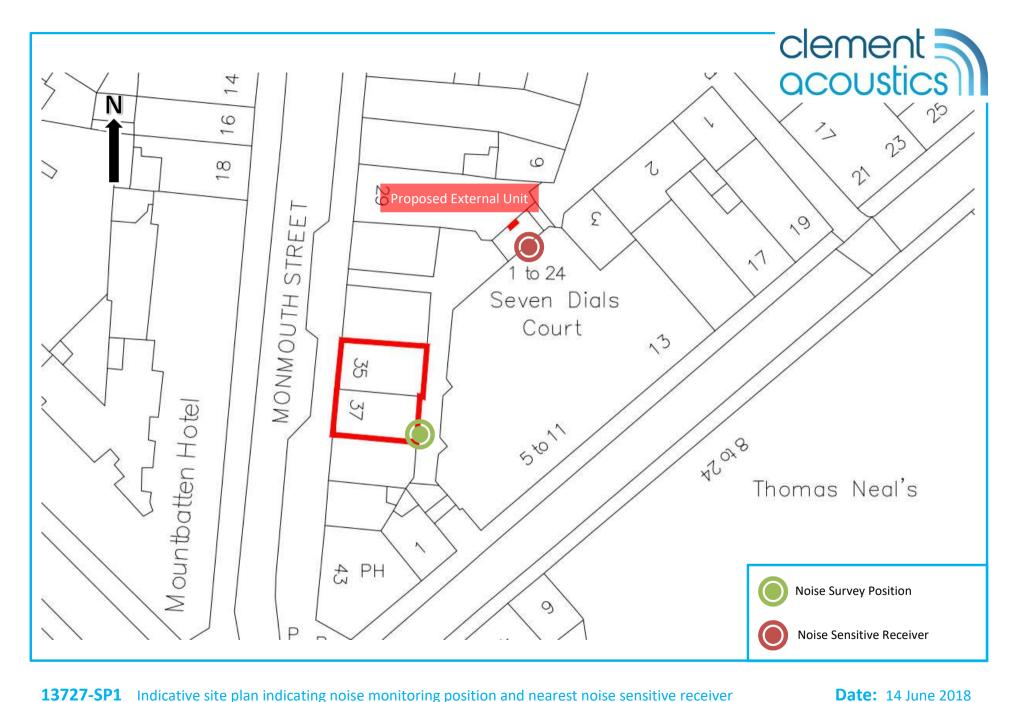
**13727-SP1** Indicative site plan indicating noise monitoring position and nearest noise sensitive receiver
