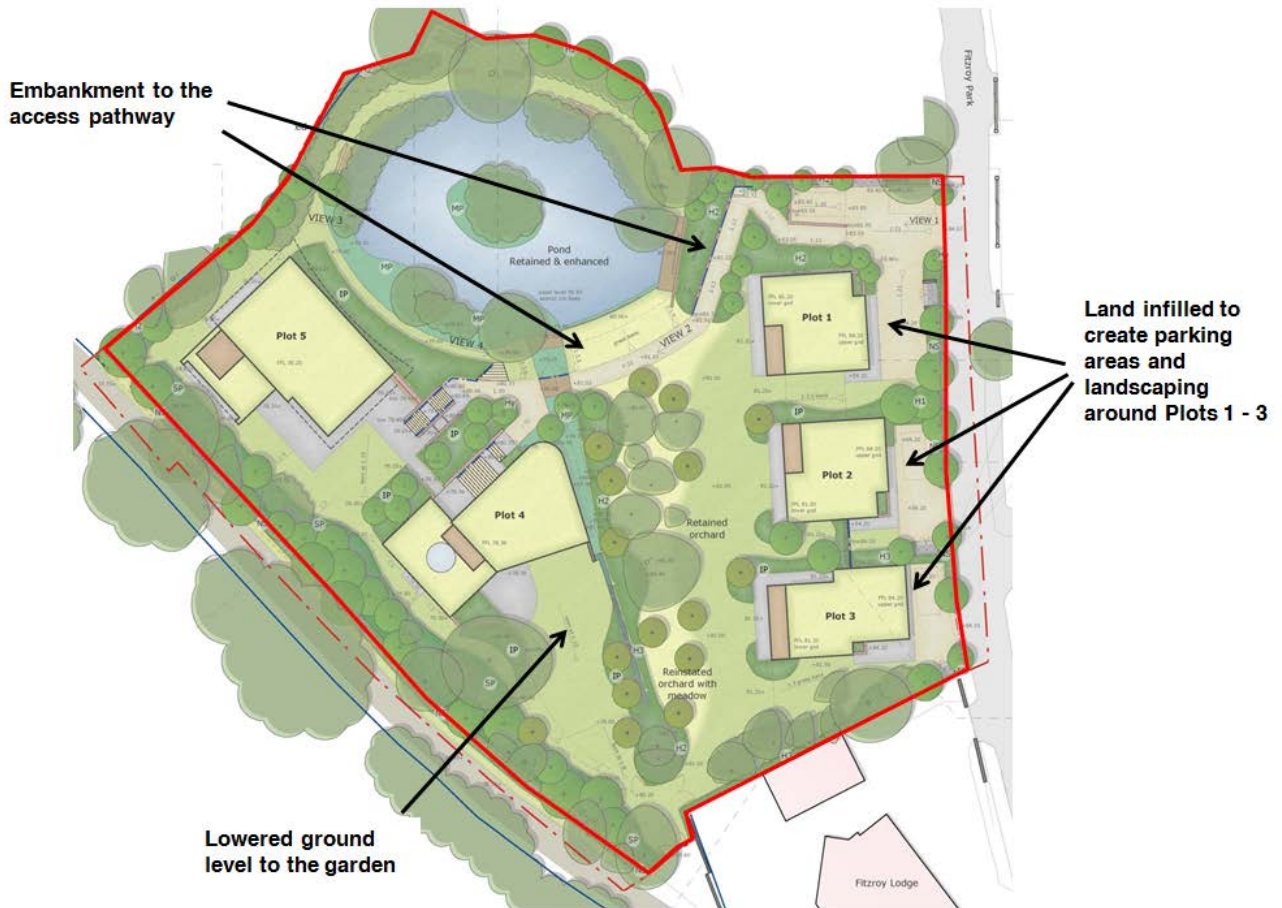
Proposed landscape plan detailing the main areas of excavation and filling as part of the development
