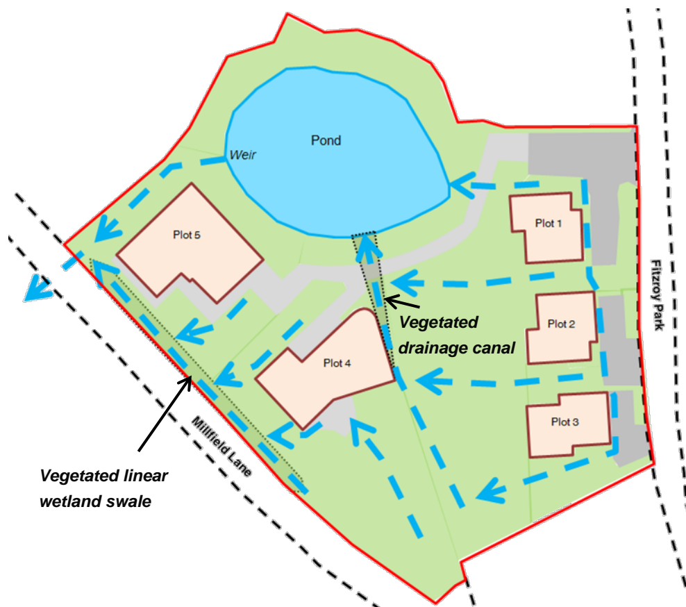
Indicative surface water drainage path directions
