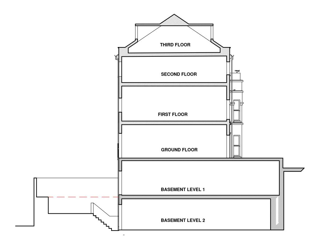
SECTION SHOWING NEW REAR BASEMENT GARDEN STAIR LEVELS AS PROPOSED
