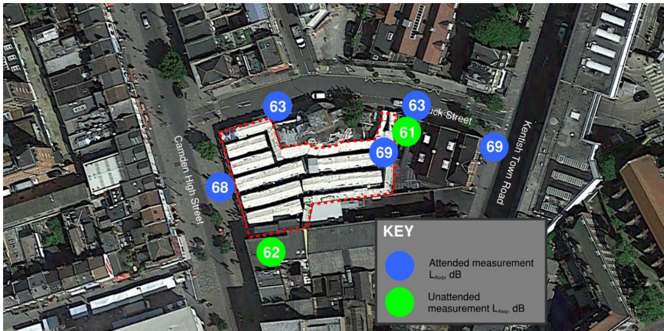
Figure 3 – Results of the acoustic survey at Camden Market
