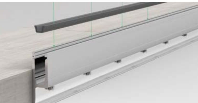
2. Insert lower glazing profile (for outdoor usage, blank out at the draining holes)
