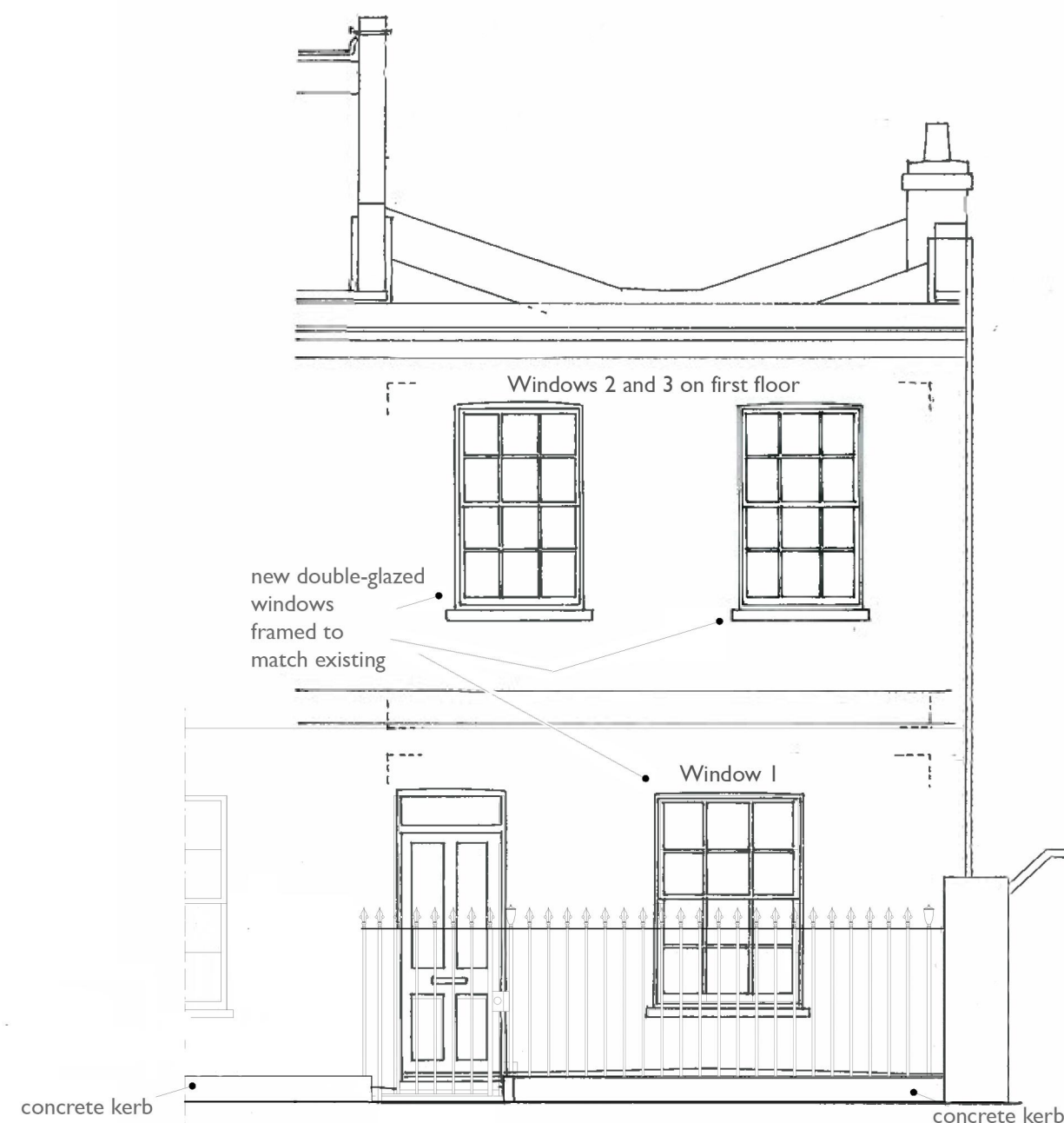
PROPOSED FRONT ELEVATION WITH RAILINGS to join the proposed railings of No 12 for which permission has been granted, and to match them in design and height Nos 14, 15, 16 have identical railings to those proposed for No 11
