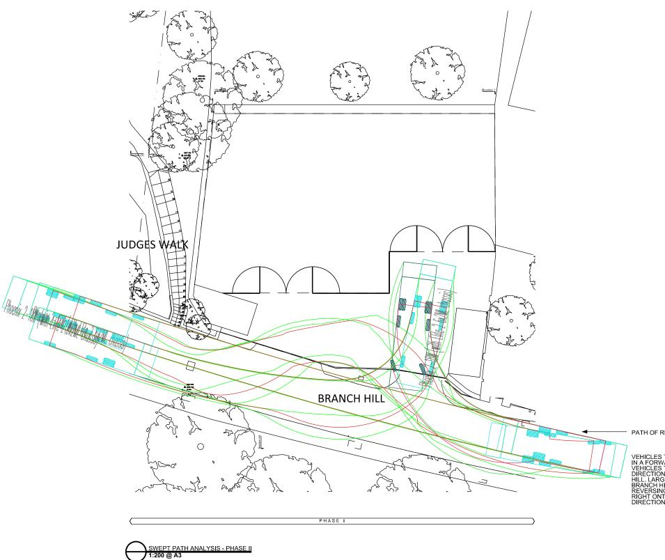
Vehicle Details: LARGE GRAB LORRY Overall Length 9.63m Overall Width 2.50m Overall Body Height 2.890m Min Body Ground Clearance 0.341m
