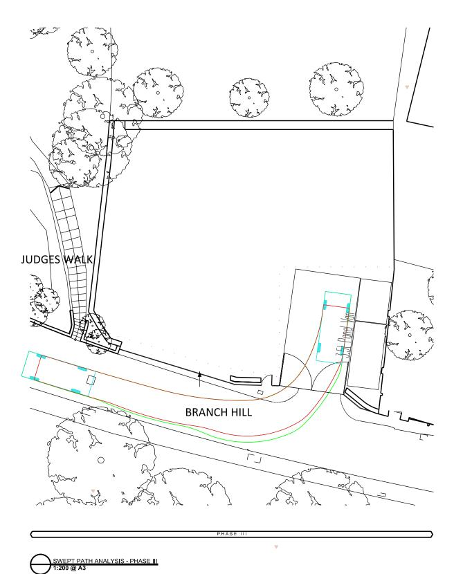
Vehicle Details: PANEL VAN Overall Length 5.245m Overall Width 1.993m Overall Body Height 2.435m Min Body Ground Clearance 0.4m
