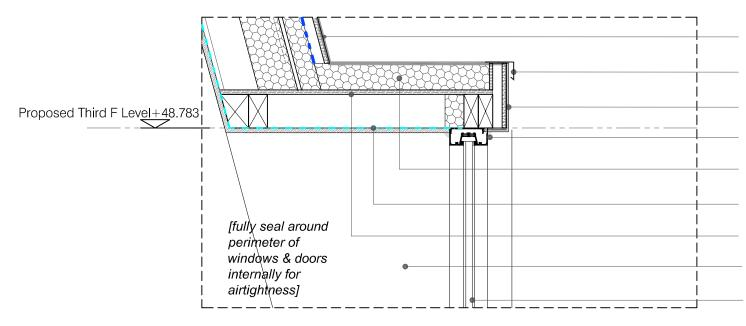
SIG Armourplan Single ply membrane (Standing seam Single Ply membrane) - colour Grey
