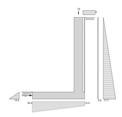
Loads shown in kN/m, pressures shown in kN/m<sup>2</sup>
