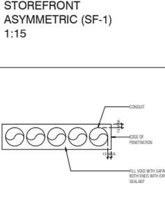
**MULTIPLE PENETRATION ACOUSTIC CONSTRUCTION**
