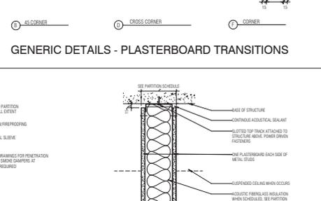
**TOP JOIN DETAIL OF PARTITION TO SLAB**
