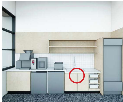
PLYWOOD DOOR FINGER PULL
