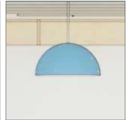
FX-05: MEETING ROOM DOME BESPOKE BLUE COLOUR SPEC TBC CONTRACTOR TO SUPPLY
