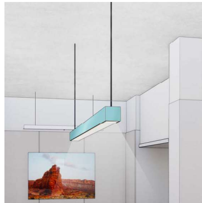
FX-08 LINEAR LIGHT IN BULE FINISH RAL 6034 SPEC TBC LENGTH: TBC CONTRACTOR TO SUPPLY
