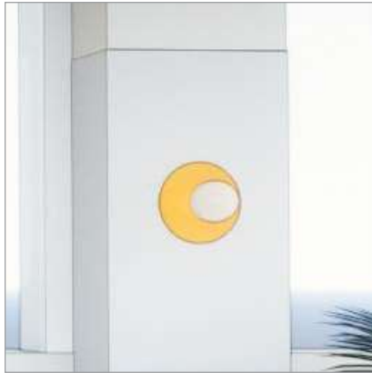
FX-12 ø300MM MDF PATRESS LACQUERED TO MATCH RAL 1003 HIGH GLOSS FINISH WITH FROSTED GLOBE BULB. CONTRACTOR TO SUPPLY MOCK UP SAMPLE REQUESTED FOR APPROVAL LAMP TO BE OFFSET OF THE WALL AND ALL THE BULB FITTING MECHANISM TO BE CONCEALED (SEE ATTACHED IMAGE)
