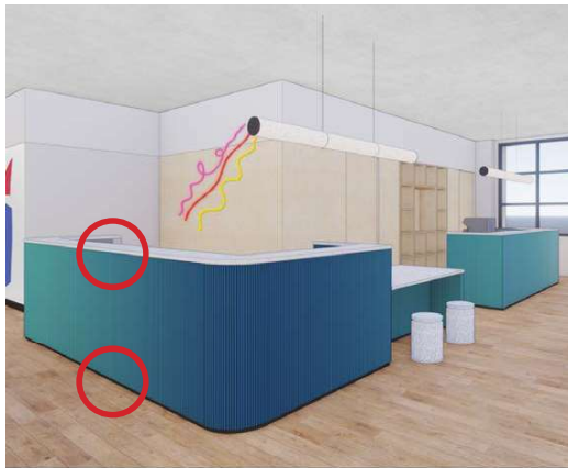
COUNTER TOP-TAMBOUR and RECESSED SKIRTING-TAMBOUR
