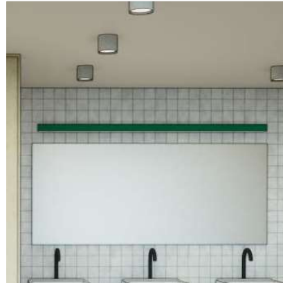
FX-13 LINEAR DOWN LIGHT IN GREEN FINISH SPEC AND COLOUR TBC LENGHT: TBC CONTRACTOR TO SUPPLY
