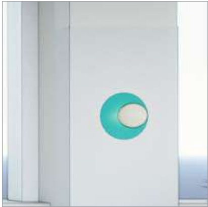
FX-11 ø300MM MDF PATRESS LACQUERED TO MATCH RAL 6034 HIGH GLOSS FINISH WITH FROSTED GLOBE BULB. CONTRACTOR TO SUPPLY MOCK UP SAMPLE REQUESTED FOR APPROVAL. LAMP TO BE OFFSET OF THE WALL AND ALL THE BULB FITTING MECHANISM TO BE CONCEALED (SEE ATTACHED IMAGE)
