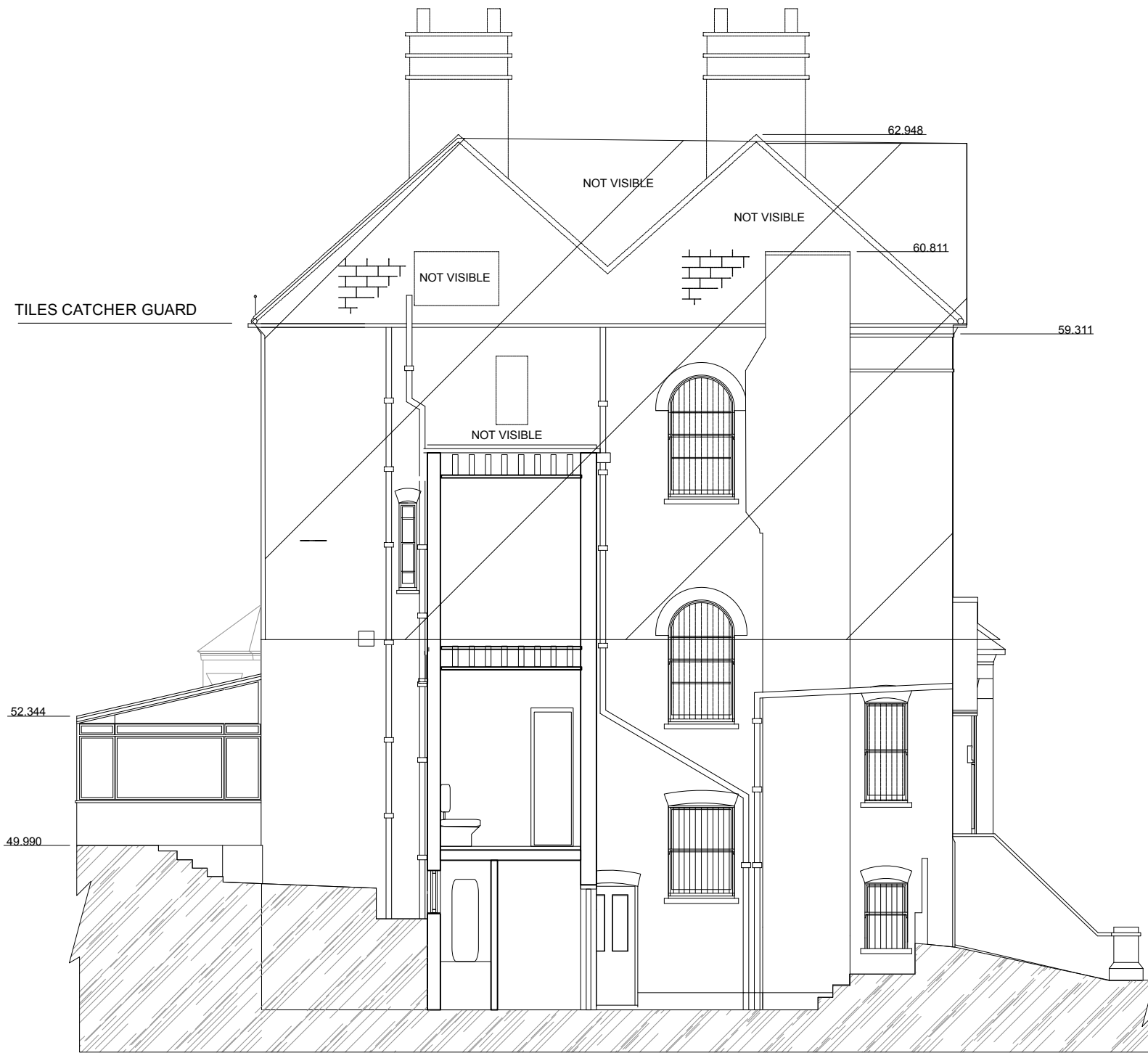
EXISTING S/W SECTION ELEVATION C-C
