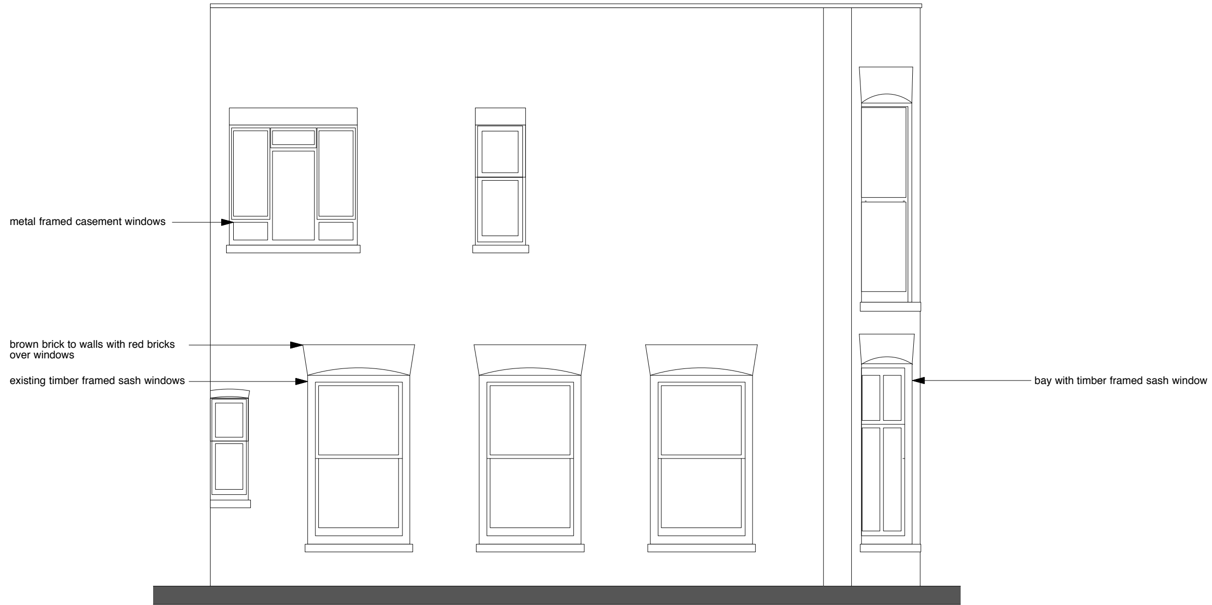
EXISTING SOUTH ELEVATION
