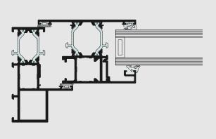
Eco system, consisting of variants Eco system 50 and Eco system 75, is a high performance aluminium system that combines aesthetic design with energy efficiency. With a Uf-value down to 2.25 W/m²K, it meets all the latest thermal insulation requirements.
