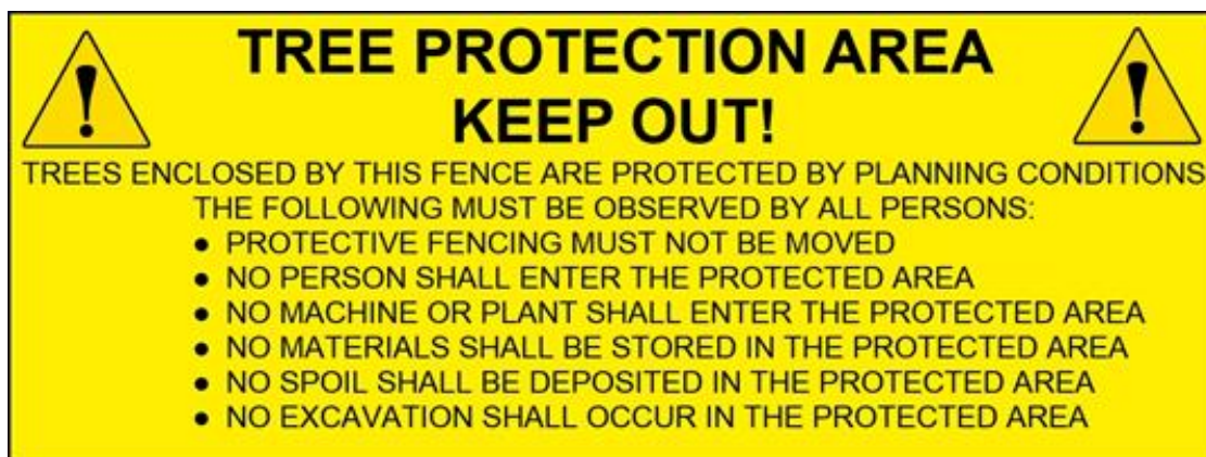
Figure 9. Wording to be included in high visibility all-weather sign attached to protective fencing
