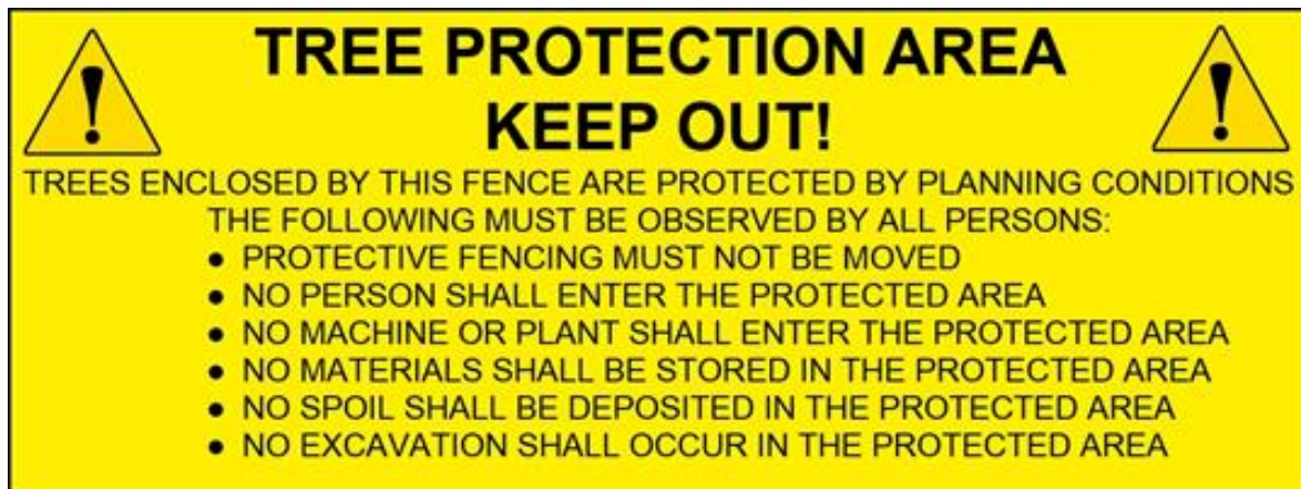
Figure 6. Wording to be included in high visibility all-weather sign attached to protective fencing
