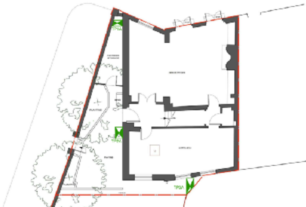
Location of trial pits to determine tree root spread
