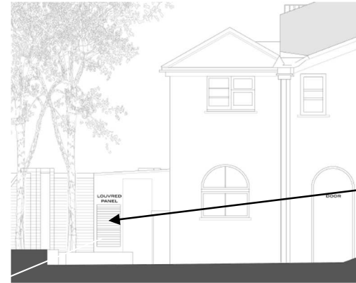
Western Elevation Showing Plant Room Louvre
