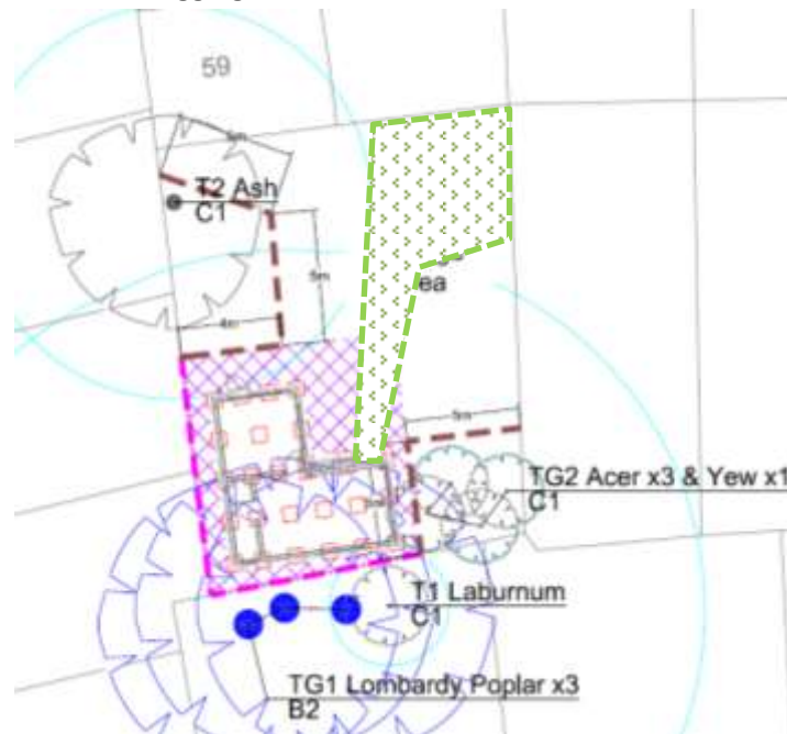
Fig 6 – A large zone (indicated above) is available for service trench installation outside retained tree RPA's
