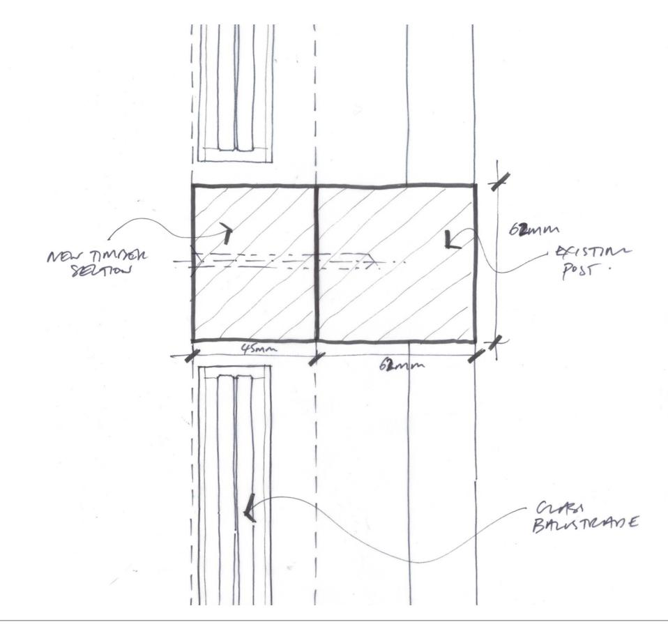
**3. Detail at vertical post** Horizontal section through post
