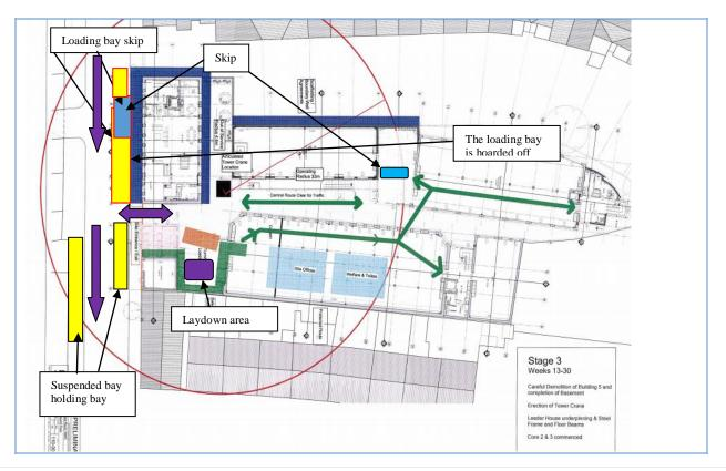
This diagram shows access onto site and the route when leaving site. Laydown areas are also shown which will move as the project progresses. We will however only ever use two number positions. The loading bay with the skip will be hoarded-off with gates at both end to allow access and egress for either side. This will prevent traffic being blocked by construction activity or construction traffic.
