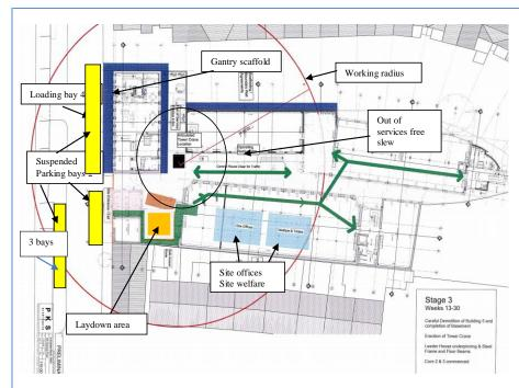
In blue we are showing a gantry scaffold which sits in front of Leeder House. We will be closing the parking bays parallel to the front of Leeder House, and will be closing the footpath in the same area.
